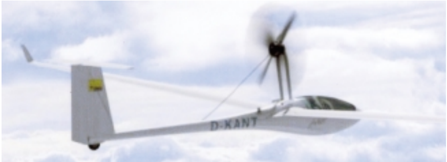
Antares can now reach 3000 m in powered flight using Saft lithium-ion batteries, as opposed to 1890 m when it used a Ni-MH system.
